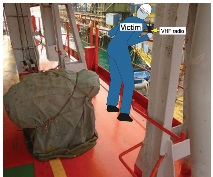
Position of victim just prior to spring line recoil
