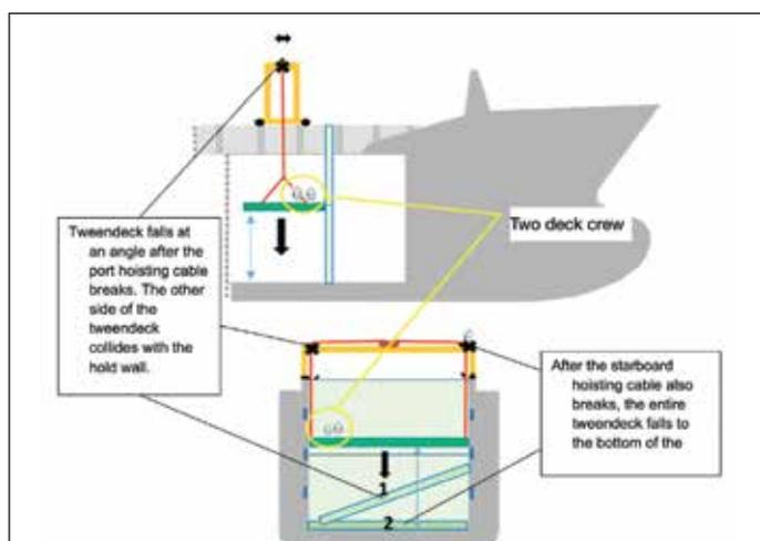
The port hoisting cable broke and the port side of the tweendeck fell to the bottom of the hold, damaging the starboard side of the hold wall and sending the two crew tumbling to one side. The starboard hoisting cable then also broke, and the entire tweendeck fell to the bottom of the hold.
